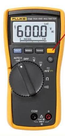
Yellow SECONDARY FUNCTION button toggles between mV ac and mV dc.
